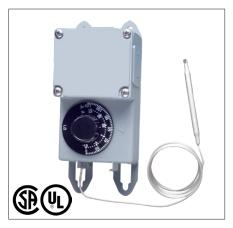
The PX thermostat is designed for temperature control applications (pipe freeze protection, roof & gutter de-icing or snow melting) in ordinary areas. The unit is housed in a weatherproof NEMA 4X enclosure. The PX thermostat can be used in an ambient-sensing mod, line sensing mode or used to control a contactor coil.
