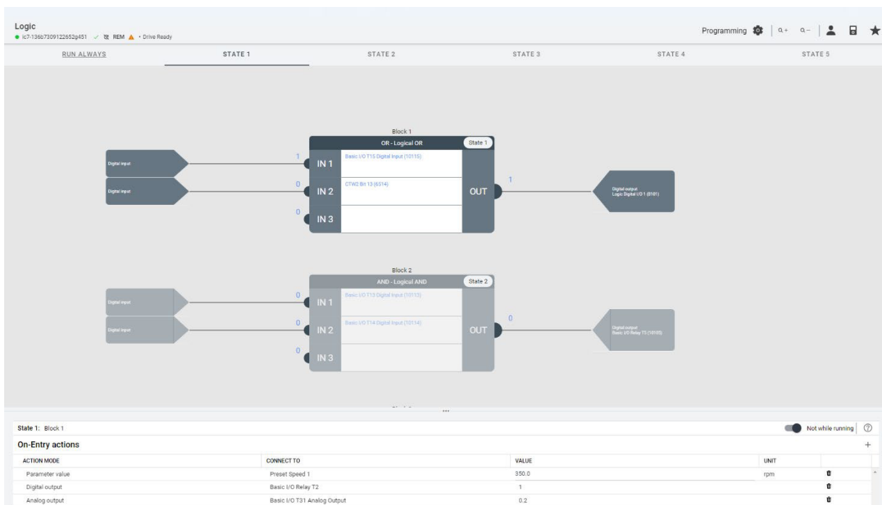
Illustration 5: Logic State 1 being edited. Function Block 1 is assigned to State 1 and only executes when State 1 is active.
