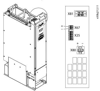
Figure 35: Auxiliary Terminals of the Power Unit
