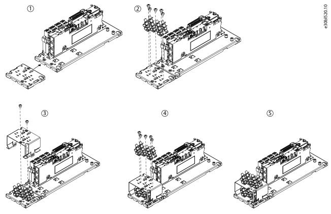
Figure 40: Assembling the Mounting Plate
