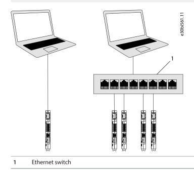
Figure 50: Connecting the Drive to a PC
