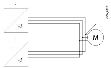
Figure 23: Recommended Installation
