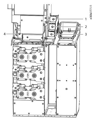
Figure 30: LCL Filter Terminals to the AFE Module
