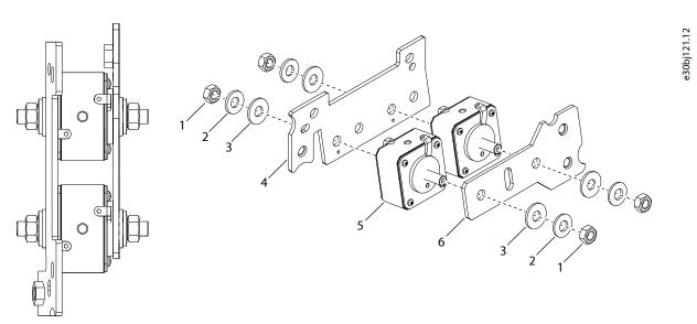
Figure 25: Installing the Fuses to the Busbars, 2 Fuses
