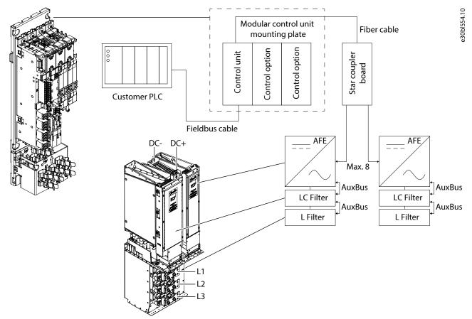
Figure 20: Example of a Control System of an AFE Module and LCL Filter
