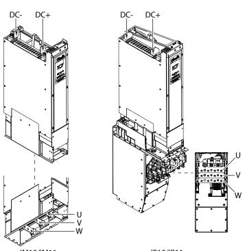
IM10/IM11 IR10/IR11 Figure 34: Locations of the Terminals on the System Modules
