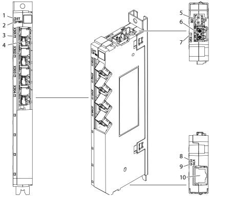
Figure 45: Terminal and Indicator Light Locations on the 4-port Star Coupler Board
