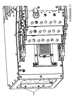
Figure 11: Bottom Screws of the Short Integration Unit, IR10, IR11
