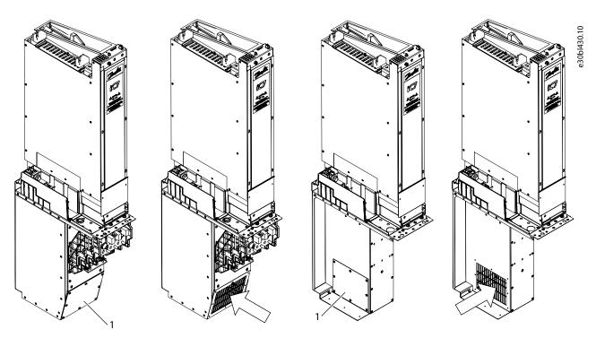
Figure 17: Removing the Air Inlet Cover for Cooling, Inverter (left) and AFE (right)
