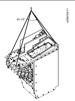
Figure 4: Lifting the Integration Unit
