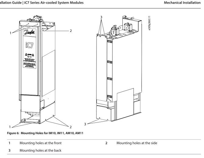
2. Attach the system module to the back wall of the cabinet and to the front mounting brackets.
