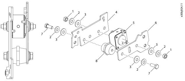
Figure 26: Installing the Fuse to the Busbars, 1 Fuse
