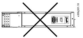
Figure 5: Forbidden Installation Direction of the System Module, Size 11
