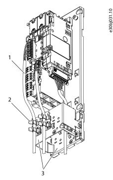
Figure 42: Example of Installing the Control Cables
