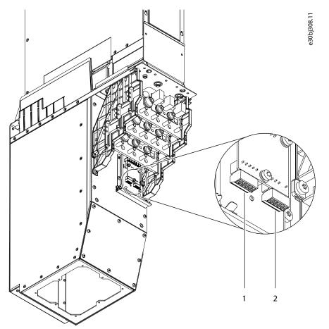
Figure 37: AuxBus Terminals of the Integration Unit with Filter
