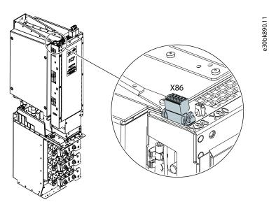
Figure 36: AuxBus Terminal of the LCL Filter (X86)
