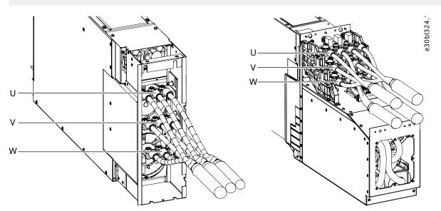
Figure 31: Motor Cable Installation, IM10, IM11 (left) and IR10, IR11 (right)
