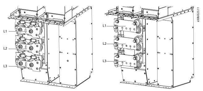
Figure 29: Mains Terminals of the LCL Filter with Fuses (left) and without Fuses (right)
