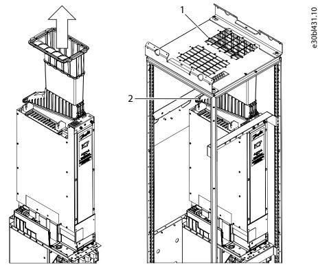
Figure 18: Outlet Airflow with or without a Top Duct
