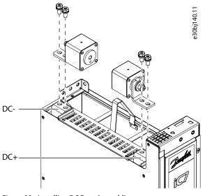
Figure 33: Installing DC Fuse Assemblies
