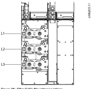
Figure 28: Filter Cable Mounting Locations
