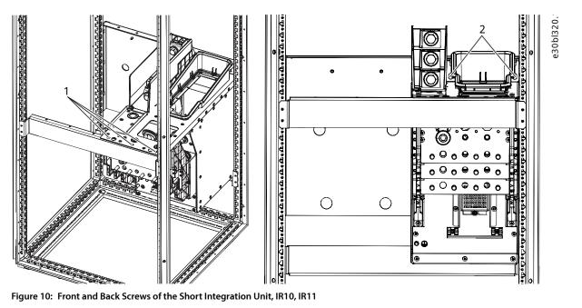
1 Mounting holes at the front 2 Mounting holes at the back
