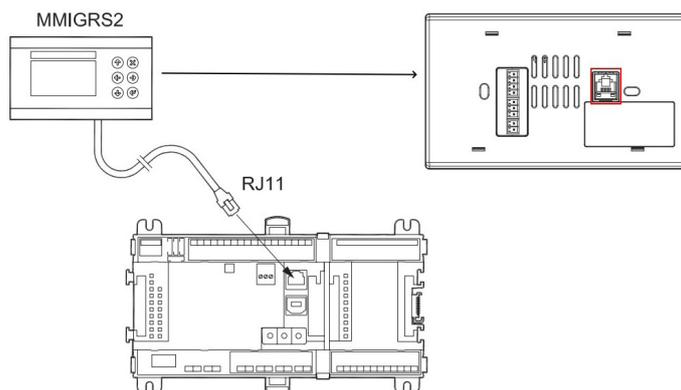
CANH-R connection should be done only on the first and last element of the network. AK-PC 78x is terminated internally and the last element of the network will be the X-Gate therefore do **not** terminate the display. Also do **not** connect a separate power supply for the display. Supply comes directly from the controller via cable.
