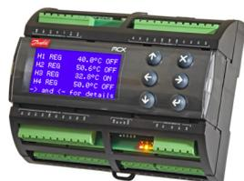
**DEVIreg™ Hotwater** is an electronic programmable controller with 4 channels for on DIN rail mounting. Every channel can be set individually to maintain hot water with the option to disinfect manually, or on a schedule. The channels sensors can be selected between 7 different temperature sensors including NTC 15 kOhm at 25°C. Building Management System (BMS) control is
