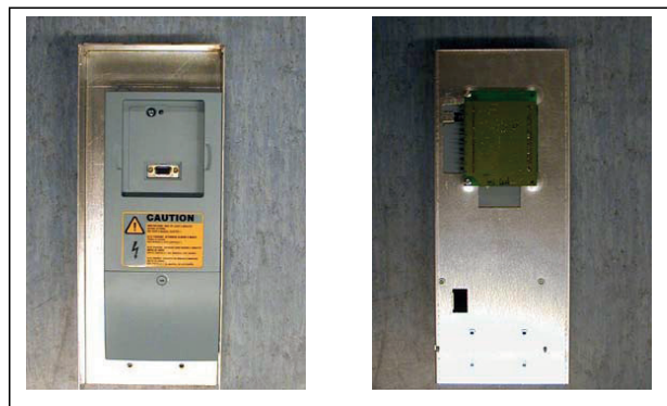
Figure 69. Control unit installed into the mounting box; Left: front; Right: back
