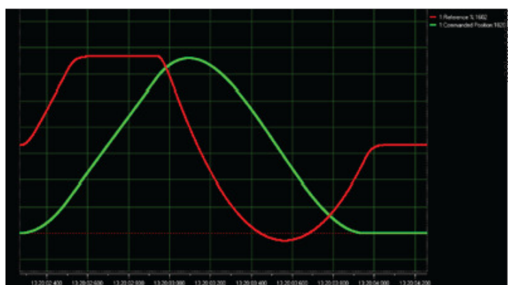
Figure 70: Follower Speed and Position
