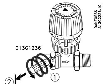
To remove the theft protection use screwdriver 013G1236 and screw into the hole (1). Pulled out until the stop is reached (2).
