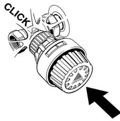
Push the thermostat firmly onto the valve until an audible "click" is heard.
