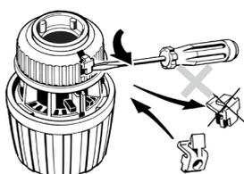
Remove the cover and install the theft protection button, code 013G5245 without pushing it all the way in.
