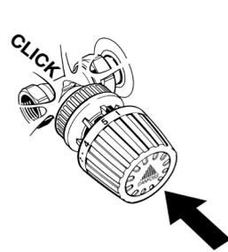
Push the thermostat firmly onto the valve until an audible "click" is heard.
