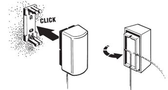
The remote sensor must not be in a drafty location or be covered. Do not install above a heat source. Attach the sensor bracket to the desired location. Pull out the required length of capillary tube and secure to the sensor as shown. Push the sensor onto the base.
