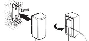
The remote sensor must not be in a drafty location or be covered. Do not install above a heat source. Attach the sensor bracket to the desired location. Pull out the required length of capillary tube and secure to the sensor as shown. Push the sensor onto the base.
