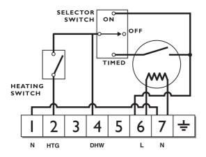
Terminals 3 and 5 are not internally connected to the programmer and may therefore be used as spare wiring terminals if required.
