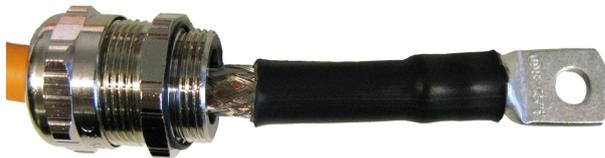
9. Insert the cable through the corresponding hole in the connection box and connect the cable lug to the connection point. Use spring washer between the cable lug and the connection screw or nut. Do not tighten the connection at this point to ensure fitting of the cable gland.
