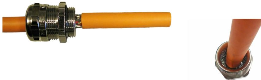
5. After the cable gland is in place remove the length A piece of the sheath and cut the braid screen (cover) from 10 mm (distance C) from the gland bottom as shown in Figure below. *Before* cutting the braid screen, verify that the cable gland spring is correctly positioned against the cable sheath, which must be protected with copper tape.
