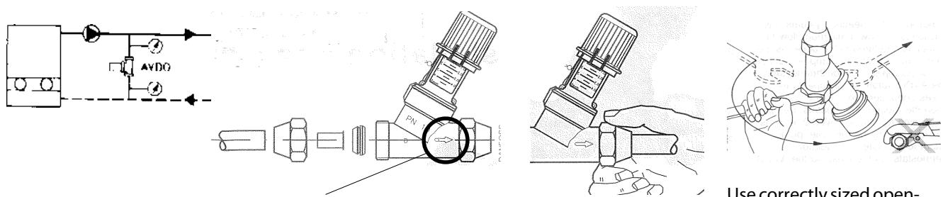
The valve should be installed in a straight run of pipe, not close to a bend.
