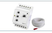
The **DEVIreg™ 316** is an simple electronic thermostat with enhanced functionality which can be installed in electric cabinets with DIN rail attachment. The thermostat is mainly used for frost protection on roofs, in gutters and downpipes. Additionaly it
