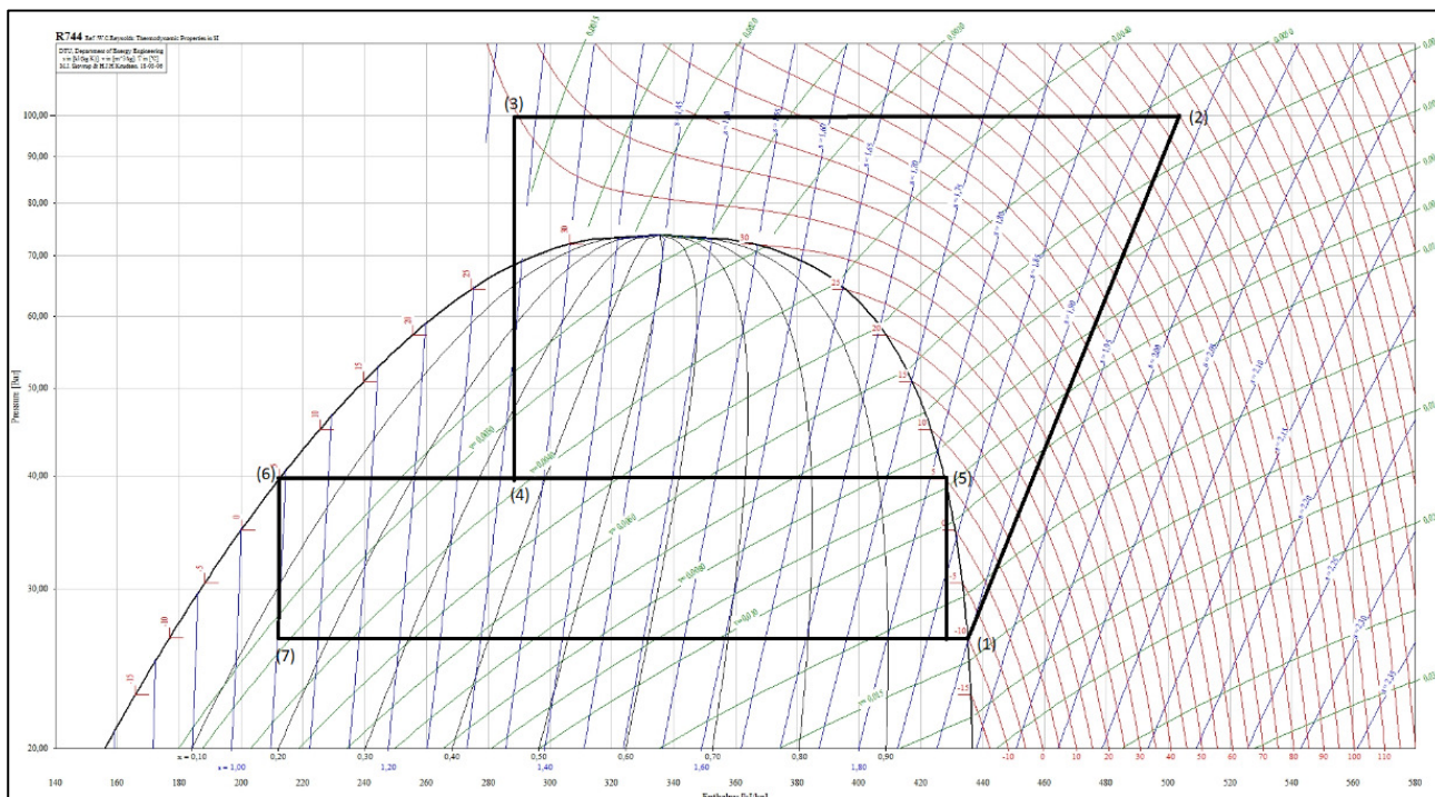
Figure 1.11 Log(p)-h diagram for a transcritical CO 2 system with intermediate pressure receiver
