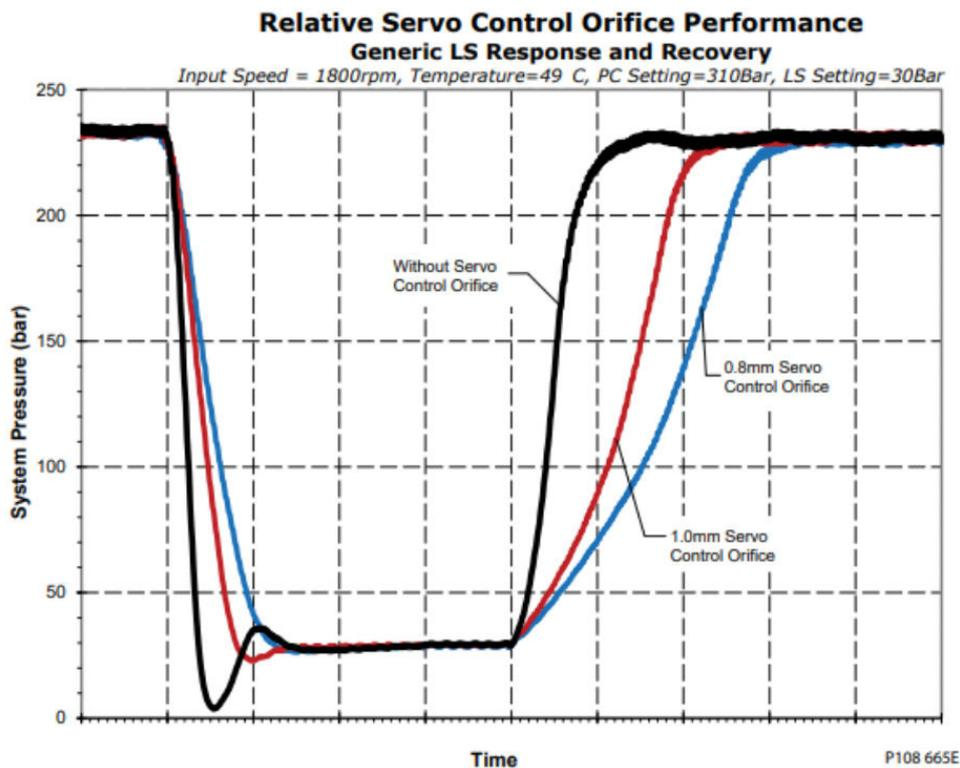
We recommend that systems experiencing instability use a Servo Control Orifice. Start with the largest size orifice available, and work down to the smaller size until the system is satisfactorily tuned. All Fan Drive systems should start with a 0.8mm Servo Control Orifice, if possible. Systems including motors are more likely to require the Servo Control Orifice option.
