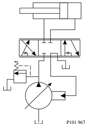
Most load sensing systems use parallel, closed center, control valves with special porting that allows the highest work function pressure (LS signal) to feed back to the LS control. Margin pressure is the difference
