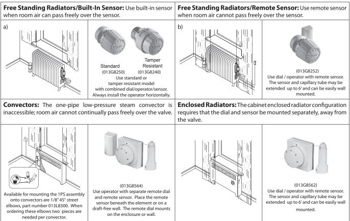
(Remote sensors are not to be placed under cast iron elements of any type)
