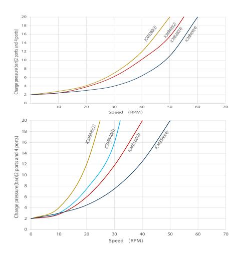
Note: Charge pressure must be maintained at the low pressure port for all types of installation.
