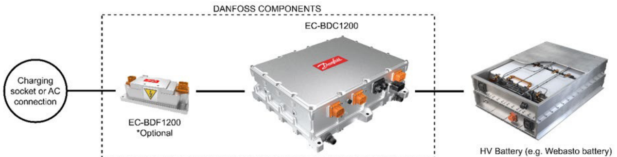
Picture 3 EC-BDC1200 application example with EMI filter EC-BDF1200-63
