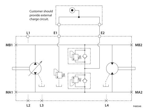
\*L1, L2, L3 and L4 are (Case) Drain ports.
