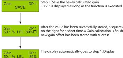
After the value has been successfully stored, a square appears on the right for a short time.= Gain calibration is finished and new gain offset has been stored with success.
