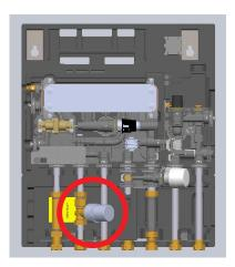
The water hammer resistor is placed at the domestic hot water supply.
