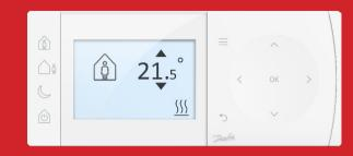
TPOne delivers new levels of user friendly interaction, the large backlit display uses easy to read icons and text information to provide feedback on status and settings to the install and user. Users can choose 24 hour, 5/2 day or 7 day programming with the option of 1, 2 or 3 heating periods. With models including, Opentherm, RF and WiFi variants, TPOne offers a solution for almost every application.
