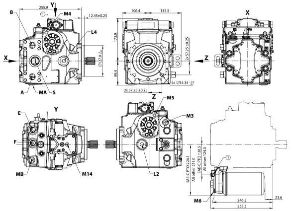
**A/B** system ports: Ø25.4–450 bar; Split flange boss per ISO 6162 **MA/MB** (system), **M3, M6** (charge) gauge ports per ISO 11926-1:  $\frac{9}{16}$ –18 **M4, M5** (servo), **M14** (case) gauge ports per ISO 11926-1:  $\frac{7}{16}$ –20 **L2, L4** – Case drain ports per ISO 11926-1:  $\frac{11}{16}$ –12
