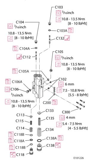
LS control shown; parts C104 through C106 and C112 through C118 are not used on PC control
