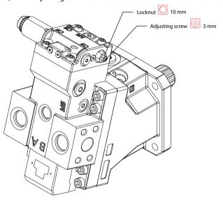
2. Use a 3mm internal hex to hold the PCOR adjusting screw in place and use a 10mm wrench to tighten the lock nut to 8 N-m [6 lbf-ft].
