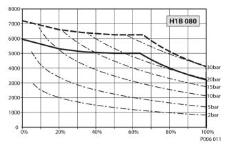
Speed (rpm) and Pressure (bar) versus Displacement (%)
