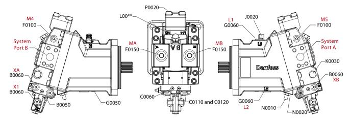
Two-position controls port, plug and fasteners (with radial ported endcap)
