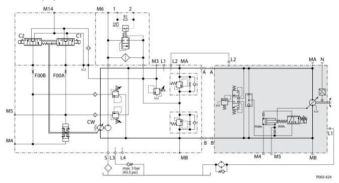
The schematic above shows the function of a hydrostatic transmission using an H1 axial variable displacement pump with electric proportional displacement control (EDC) and an H1 bent axis variable displacement motor with electric proportional control (L\*) and integrated loop flushing device.
