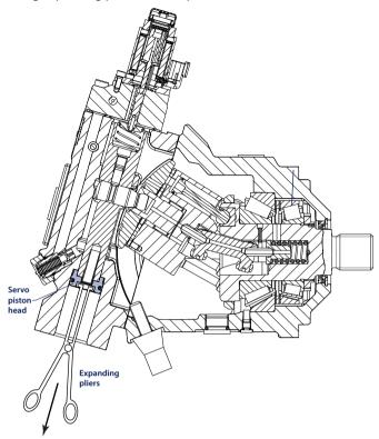
6. Remove and discard seal ring (P0044) and O-ring (P0043).
