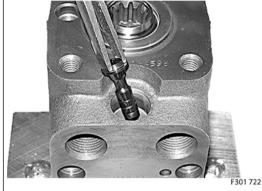
Install the spring (31) on top of the piston (32).
