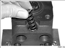
Place o-ring (43) on adjusting screw (30). Screw in the adjustment screw (30) with a 6 mm Allan key. Make the pressure setting on a test panel according to valve setting specification.
