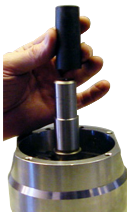
21. Mount the tool over the shaft.
