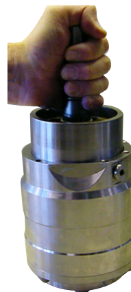
8. Mount the cylinder barrel in the housing.
