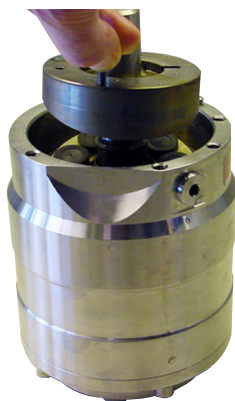
7. Remove the swash plate using the front screw.
