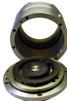
10. Separate the housing and the end cover.
