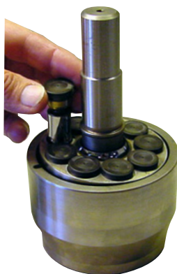
13 Remove the pistons.
