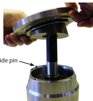
22. Mount the front flange on the housing using the pin as guide. 23. Remove the tool.
