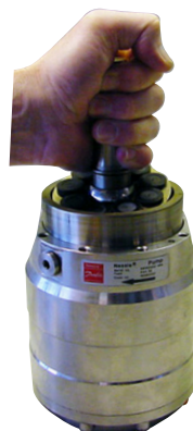
8. Remove the cylinder barrel from the housing.
