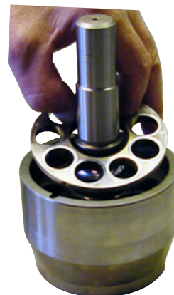
14. Remove the retaining plate.
