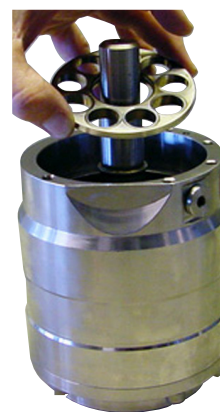
10. Mount the retaining plate (smallest centre diameter pointing upwards).
