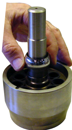
15.Remove the retaining ball.
