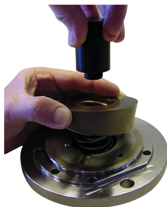
17. Press the swash plate against the flange and screw the tools together.
