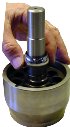
15.Remove the retaining ball.
