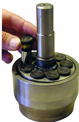
13 Remove the pistons.
