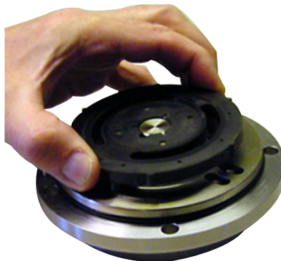
11. Remove the valve plate from the end cover.
