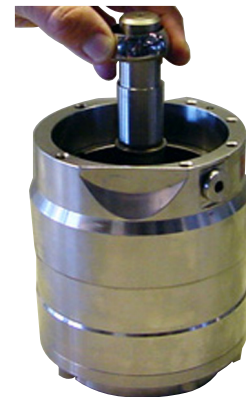
10. Slide the retaining ball (smallest diameter pointing upwards) down the shaft.
