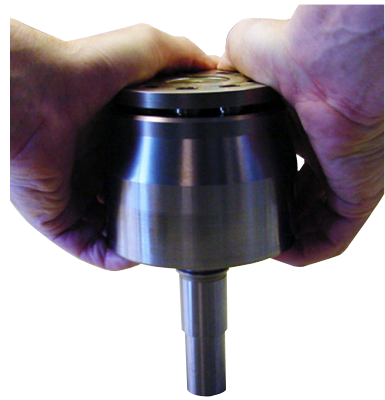
8. Press the thrust plate into the cylinder barrel using a table or the like as support.
