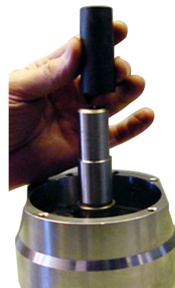
22. Mount the tool over the shaft.
