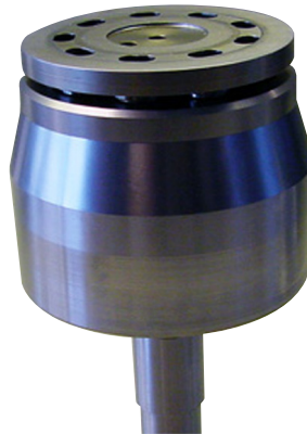
7. Mount the thrust plate with sealings on the cylinder barrel.
