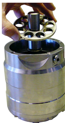
11. Mount the retaining plate (smallest centre diameter pointing upwards).
