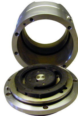
10. Separate the housing and the end cover.
