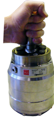
8. Remove the cylinder barrel from the housing.
