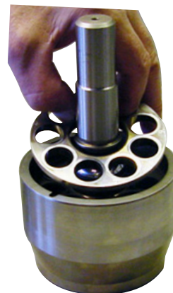
14. Remove the retaining plate.
