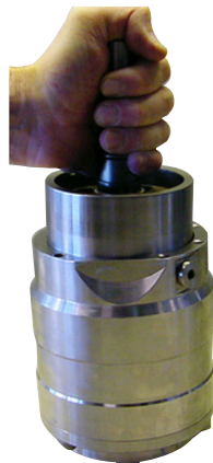
9. Mount the cylinder barrel in the housing.
