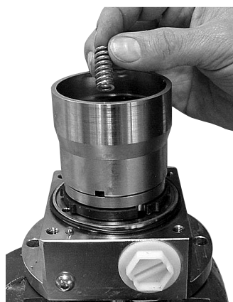
9.2.a. Mount the spring in the centre hole.
