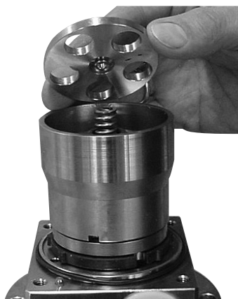
9.1.c. Mount the retainer plate.
