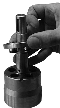
12. Remove the valve plate.
