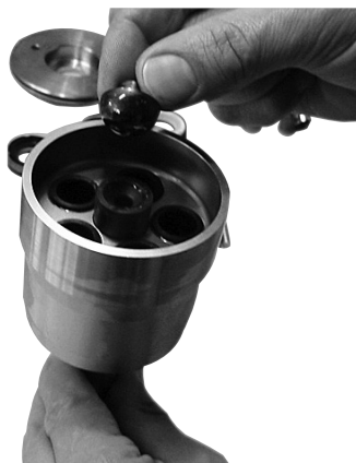
10.2.a. Remove the retainer guide.
