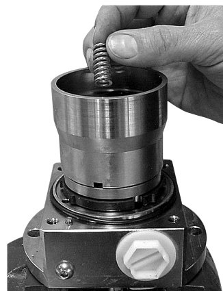
9.1.b. Mount the spring in the centre hole.
