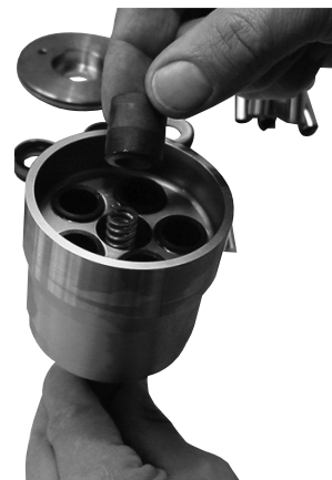
10.2.b. Remove the spring guide.
