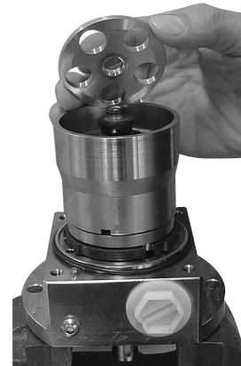
9.2.d. Mount the retainer plate on the retainer guide.
