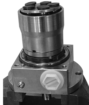
11. All pistons inserted.
