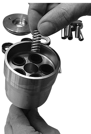
10.2.c. Remove the spring.
