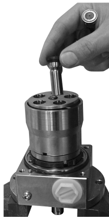
10. Insert the pistons.
