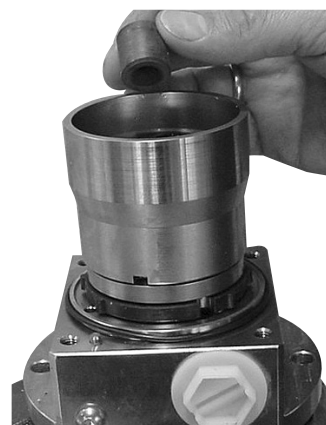
9.2.b. Mount the spring guide.
