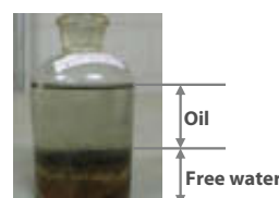
Free water in oil (Evaporator leak)
