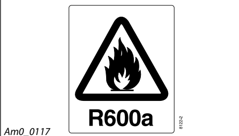
Fig. 6: Label on compressor for R600a
