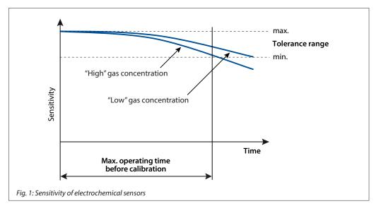
They are very accurate (+/- 2%) and tend to be used mainly for toxic gases, which cannot be detected otherwise, or where high levels of accuracy are needed (fig. 1).
