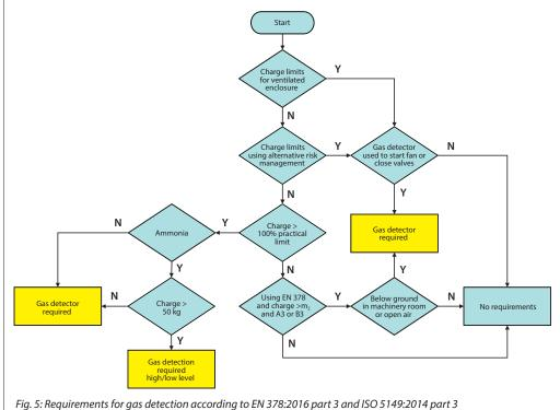
With a few exceptions gas detection is required by EN 378:2016 and ISO 5149:2014 for all installations where the concentration in a room may exceed the practical limit for that space.
