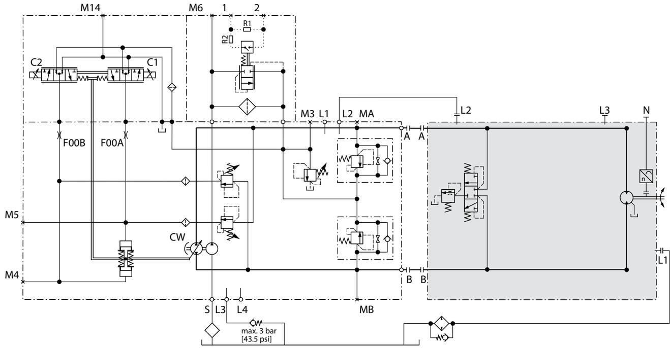
The schematic above shows the function of a hydrostatic transmission using an H1 axial variable displacement pump with electric proportional displacement control (EDC) and an H1 fixed displacement motor with integrated loop flushing device.
