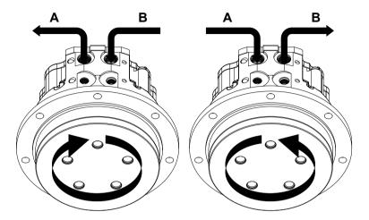
The THORX motors are based on a bidirectional design which provides the same performance in clockwise rotation as counterclockwise rotation. This provides a clear benefit in drivetrain solutions where the motor needs to reverse and don't go down in performance.
