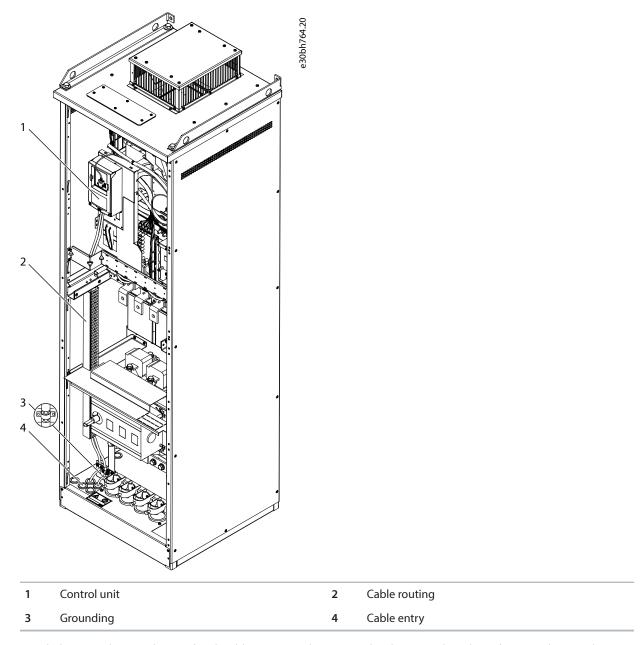
**c.** Attach the grounding conductor of each cable to a grounding terminal with a grounding clamp for grounding conductor.
