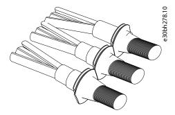
2. Attach the grommet and the cable until the frame of the drive goes into the groove of the grommet.
