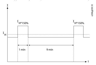
Figure 94: High Overload
