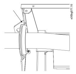
Figure 48: Rubber Grommets
