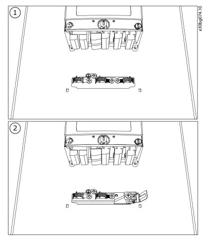
Figure 45: Attaching the Grounding Clamps for Control Cable
