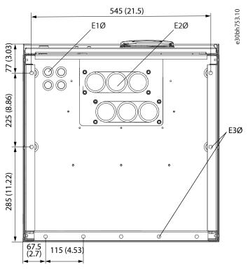
Figure 90: Dimensions of the Mounting Holes for VACON® NXS/NXP AC Drive, FR10 Standalone
