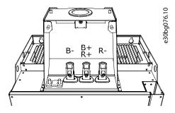
Figure 31: DC Terminals and Brake Resistor Terminals
