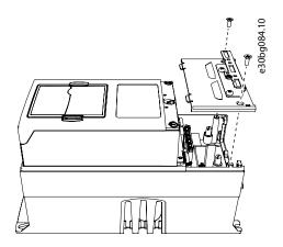
Figure 21: Opening the Cable Cover
