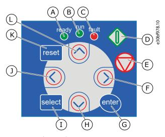
Figure 2: Keypad Buttons for VACON® NXP
