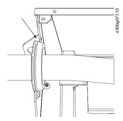
3. To make a 360° connection with the grounding clamp for cable shield, expose the shield of motor cables.
