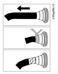
3. To achieve EMC class C1 and C2, use an EMC cable gland as an alternative to the grommet.
