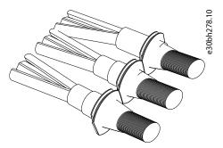
Figure 42: Putting the Cables through the Grommets
