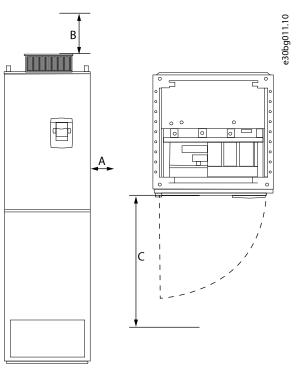
Figure 13: Minimum Clearances around the AC Drive
