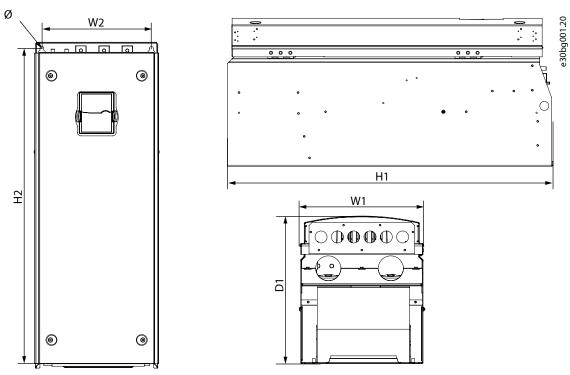
Figure 76: Dimensions of the VACON® NXS/NXP AC Drive, FR8, IP21/IP54
