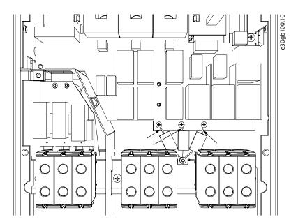
5. Remove the screw and the capacitor assembly.
