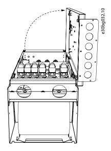
Figure 30: Opening the Power Unit Cover
