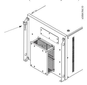
Figure 8: The Cabinet Door Key Location at Delivery
