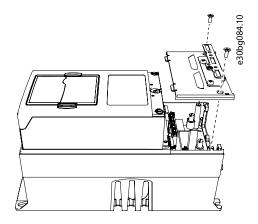
Figure 27: Opening the Cable Cover
