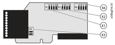
Figure 61: Jumper Blocks on OPTA1
