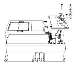
Figure 24: Opening the Cable Cover
