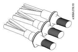
Figure 47: Putting the Cables through the Grommets
