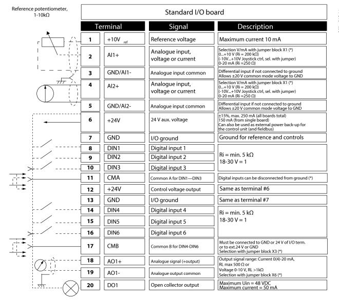
Figure 58: Control Terminal Signals on OPTA1
