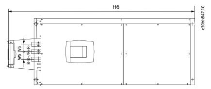
Figure 80: Dimensions of the VACON® NXS/NXP AC Drive, FR9 with DC Extension Connection Box
