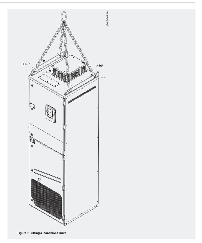
3. After lifting the drive, check for signs of damage on the drive.
