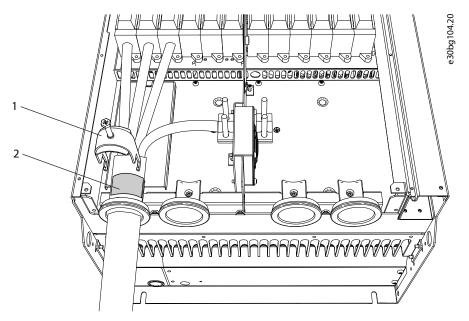
Figure 49: Exposing the Shield of the Cables
