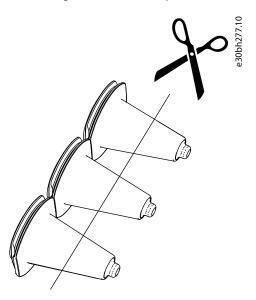
Figure 46: Cutting the Grommet in IP54
