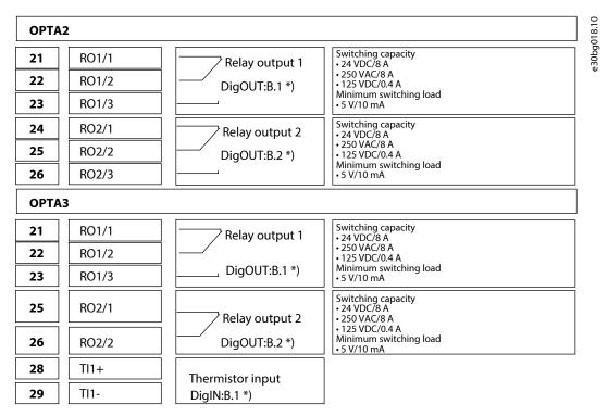
Figure 63: Control Terminal Signals on Relay Boards OPTA2 and OPTA3
