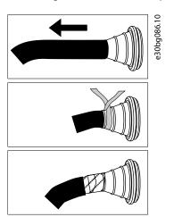
3. To achieve EMC class C1 and C2, use an EMC cable gland as an alternative to the grommet.
