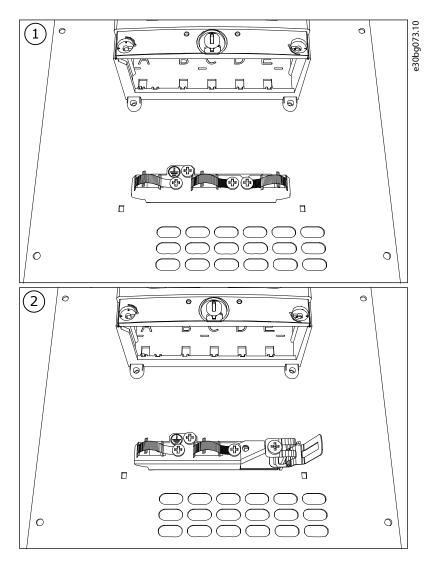
Figure 40: Attaching the Grounding Clamps for Control Cable
