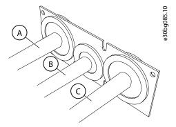
Figure 38: Cables through the Cable Entry Plate
