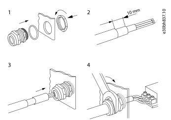
**4.** Put the cables - the DC supply cable, the motor cable, and the optional brake cable - in the openings of the cable entry plate. Use the cable entry plate delivered in the accessories bag.
