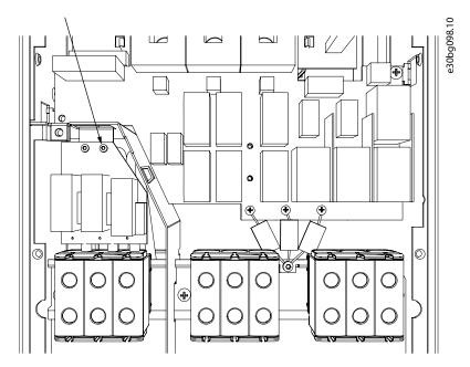
3. Remove the screw and replace with a plastic screw M4.
