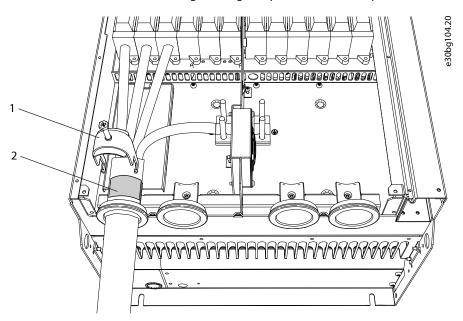
Figure 44: Exposing the Shield of the Cables
