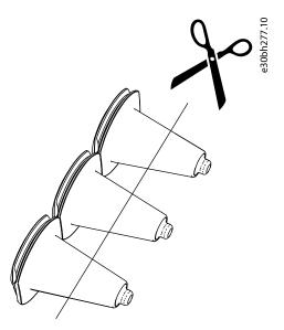
Figure 41: Cutting the Grommet in IP54
