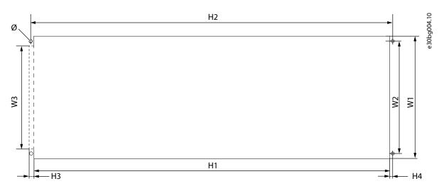
Figure 83: The Dimensions of the Opening and Drive Outline with Flange, FR4–FR6  $\,$
