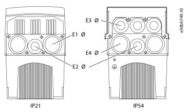
Figure 73: Dimensions of the Mounting Holes for VACON  $^{\circ}$  NXS/NXP AC Drive, FR4–FR6
