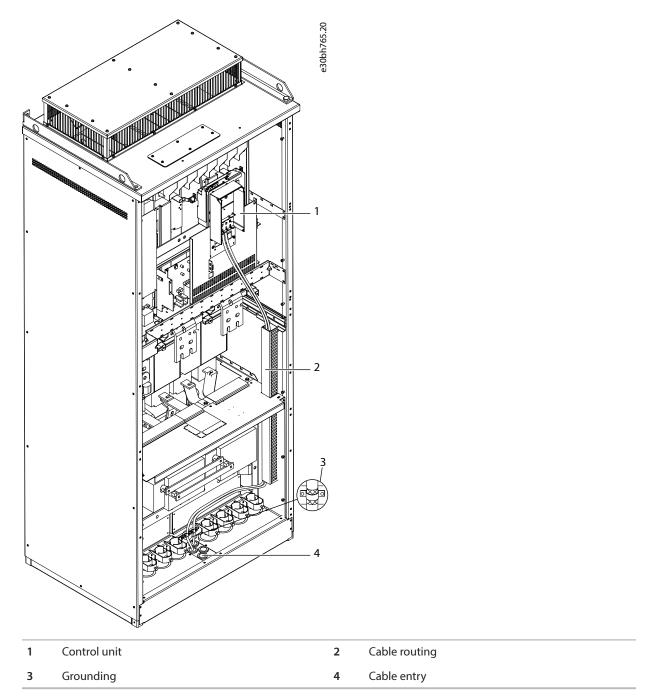
**c.** Attach the grounding conductor of each cable to a grounding terminal with a grounding clamp for grounding conductor.
