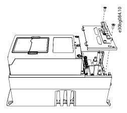
Figure 18: Opening the Cable Cover
