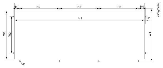
Figure 85: Dimensions of the Opening and Drive Outline with Flange, FR7
