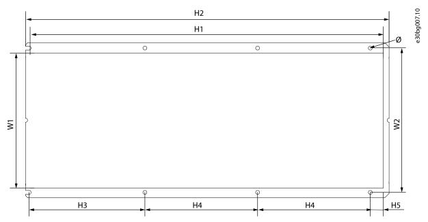
Figure 86: Dimensions of the Opening and Drive Outline with Flange, FR8
