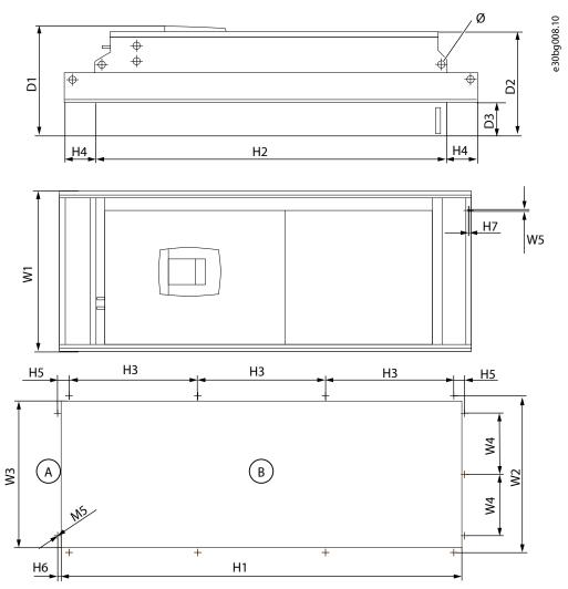
Figure 87: Dimensions of the VACON® NXS/NXP AC Drive, FR9
