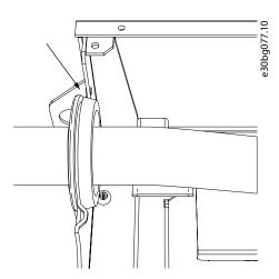
Figure 43: Rubber Grommets
