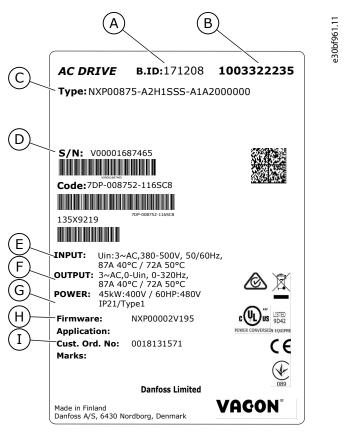
Figure 1: Package Label of VACON® NX AC Drives (Example)
