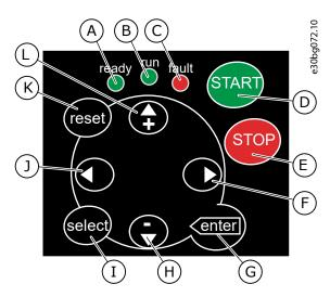
Figure 3: Keypad Buttons for VACON® NXS
