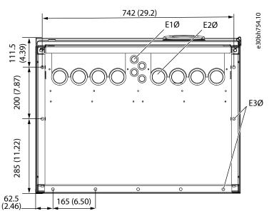
Figure 91: Dimensions of the Mounting Holes for VACON® NXS/NXP AC Drive, FR11 Standalone
