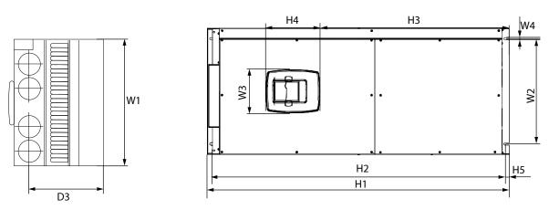
Figure 79: Dimensions of the VACON® NXS/NXP AC Drive, FR9, IP21/IP54
