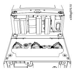
**10.** Attach the cover of the drive. For the tightening torques of the screws, see <u>12.5 Tightening Torques for Cover Screws</u>. Make sure that the control cables or the cables of the AC drive are not caught between the frame and the cable cover.
