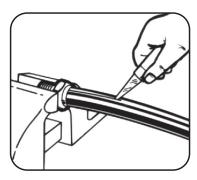
Step 1 Slit hose lengthwise from edge of coupling body to end of the barb.
