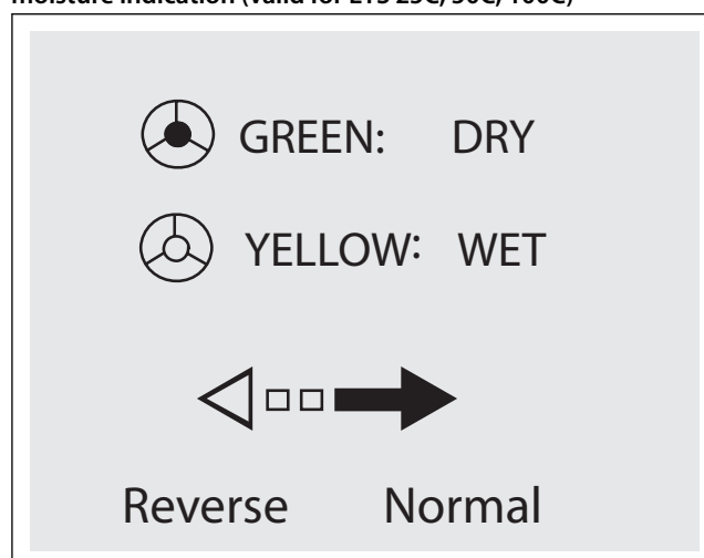
Figure 8: Laser engraved data - flow direction and moisture indication (valid for ETS 25C, 50C, 100C)
