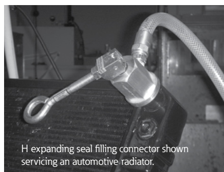
The H, K, and Connecto-Valve seal expansion is adjustable.
