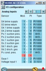
The selected module and point numbers for **Sc3 Air on** are shown in a red field instead of a blue one.
