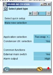
Quick setup consists of a number of settings that are all based on a system with two evaporators and one condenser.
