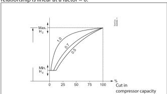
Min. and Max. frequency to be set for both the controller and the frequency converter.
