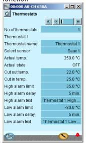
In our example we select one thermostat function for monitoring the plant room temperature.
