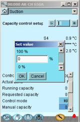
If you need to manually adjust the capacity of the compressors, you can use the following procedure:
