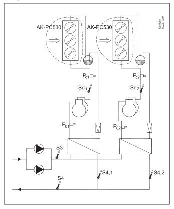
If the condenser side requires a complete control of a dry cooler circuit, AK-CH 650A can be combined with a dry cooler control, type AK-PC 420.
