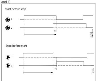
Using this setting there can be alternation between the two pumps so that a type of operating time equalisation is achieved. The period between the pump changeovers can be set as "Pump-Cycle". On changeover to the second pump, the first one will remain in operation for the "PumpDel" time. It will then stop. At stop before start "PumpDel" will be the break time for changeover.
