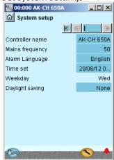
All system settings can be changed by pressing in the blue field with the setting and then indicating the value of the required setting.
