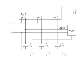
n the configuration of the controller's outputs it will be the output "FanA1‴ that will start and stop the frequency converter.
