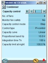
Used in our example are four step-controlled fans.
