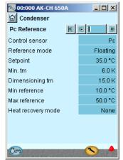
In our example the condenser pressure is controlled on the basis of the outdoor temperature (floating reference).
