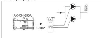
The controller can supply a 0-10 V signal, which indicates the desired speed of the pump. The signal is connected to a frequency converter.
