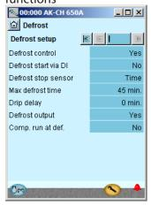
When no input is used to start a defrost cycle, this allows use of a schedule where the defrost startup times are specified. The schedule is located under the daily user interface. See page 72.
