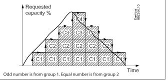
Cut-out of the last compressor stage:
