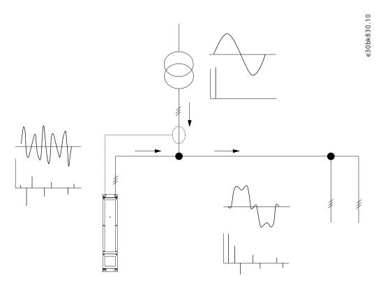
The filter sets different Silicon Carbide (SiC) switches in real time feeding a DC voltage into the grid, which creates counterphase signals. A built-in line filter smooths the compensated current waveform, ensuring that the MOSFET switching frequency and DC component is not imposed to the grid. The filter can operate on generator or transformer supply and can reduce individual motor loads, non-linear loads, or mixed loads. Consider protection for non-linear loads.
