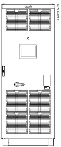
Figure 6: Example of Cabinet Integration of a 440 A Filter
