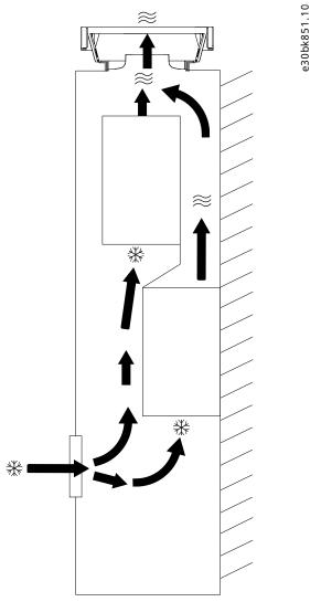
Figure 7: Airflow Considerations when Modules are Installed Above Each Other
