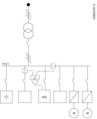
Figure 28: Capacitor Bank Mounted on PCC
