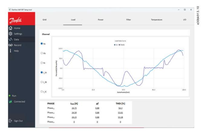
Figure 35: Load Voltages and Currents (Only Phase A Visualized)
