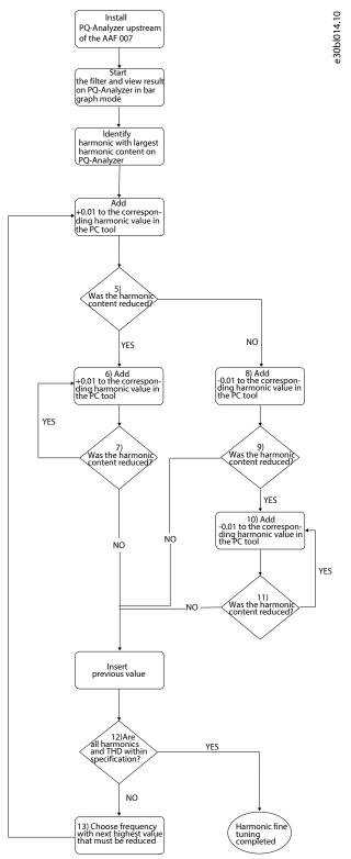
Figure 33: Flowchart of Harmonic Fine-tuning
