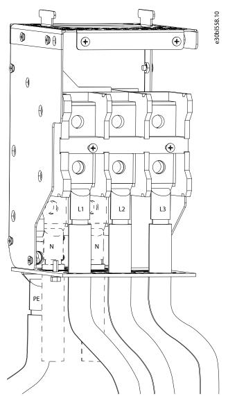
Figure 9: Mains and PE Connection for 150 A Module
