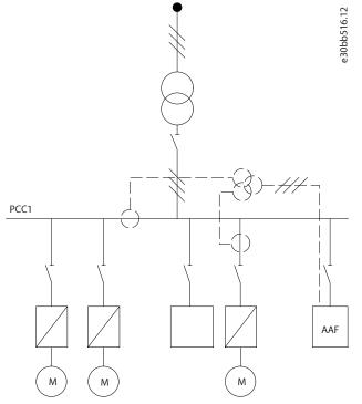
Figure 19: Selected Load Compensation in Open-loop Configuration
