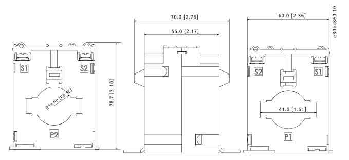
Figure 22: Dimensions, Current Transformers with Primary Current of 250 A, 400 A, 600 A, and 800 A
