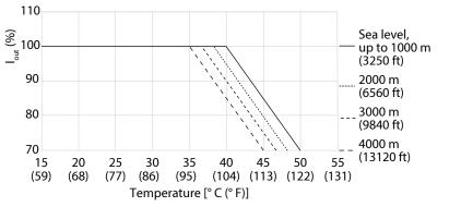
Figure 3: Derating for Temperature and Altitude
