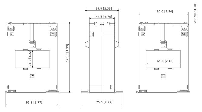
Figure 23: Dimensions, Current Transformers with Primary Current of 900 A, 1000 A, and 2000 A
