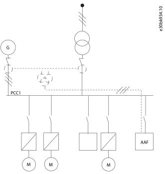
Figure 18: Multi Power Source Infeed in Close-loop Configuration
