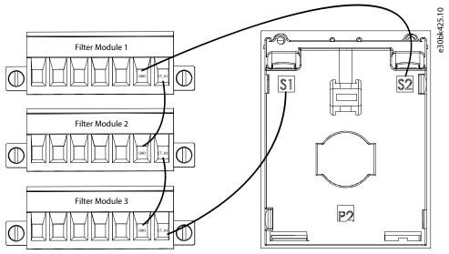
Figure 16: Wiring of a Current Transformer to 3 Filters in Series
