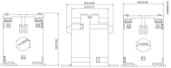
Figure 21: Dimensions, Current Transformers with Primary Currents of 80 A and 150 A
