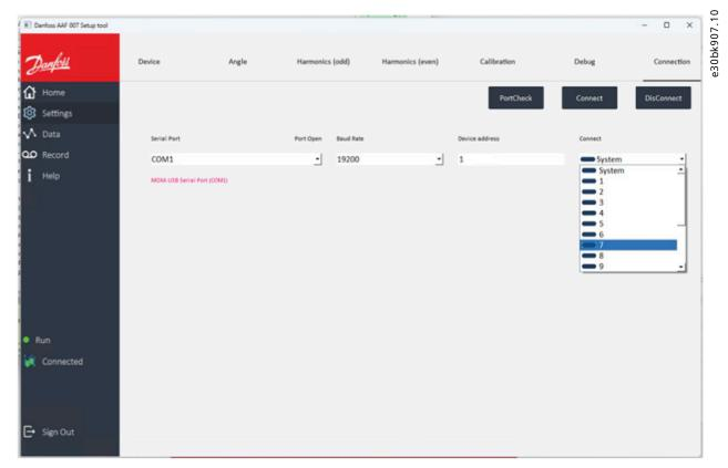
Figure 30: Selection of Filter Module and Address
