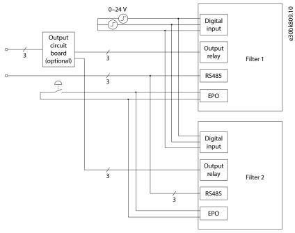
Figure 40: Example of Control Wiring for 2 Filter Modules
