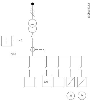
Figure 25: Capacitor Bank Mounted Upstream - Current Transformers do not Measure Capacitor Current
