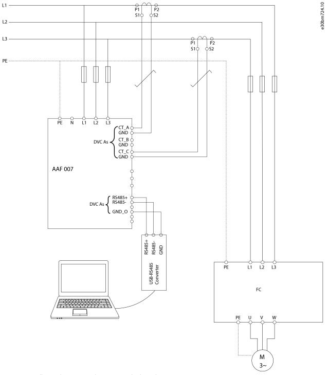
Figure 10: Installation of Current Transformers on Load-side Configuration/Open Loop
