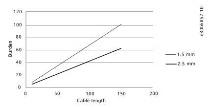
Figure 17: Burden Requirement for 1.5 and 2.5 mm Cable
