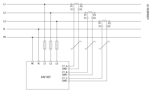
Figure 14: Four-wire Configuration
