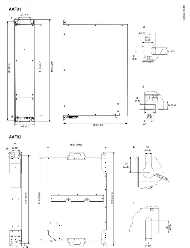
Figure 4: Mechanical Housing of AAF01 (35 A and 55 A) and AAF02 (100A and 150A) Modules
