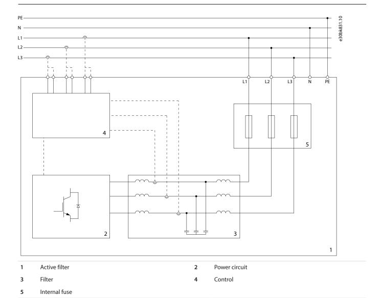
Different priorities on the compensation modes can be selected for the filter. In harmonics only (H), the full capacity is utilized to reduce the harmonic current content of the mains at the connection point up to the 60th order. In harmonic and reactive power mode (HR), all capacity that is not used for harmonic current mitigation will be utilized for reactive power compensation on the fundamental, either a fixed value for VA or towards a programmed displacement factor.
