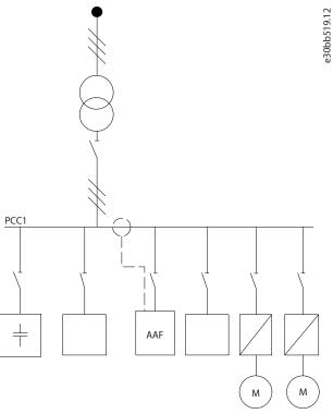
Figure 27: Current Transformers do not Measure Capacitor Current
