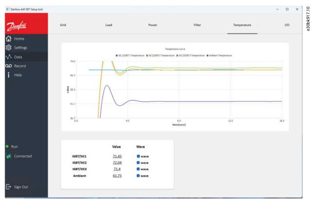
Figure 38: Temperature Values of Switching Devices in the Filter
