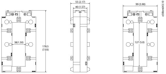
Figure 24: Dimensions, Current Transformers with Primary Current of 2500 A and 3000 A
