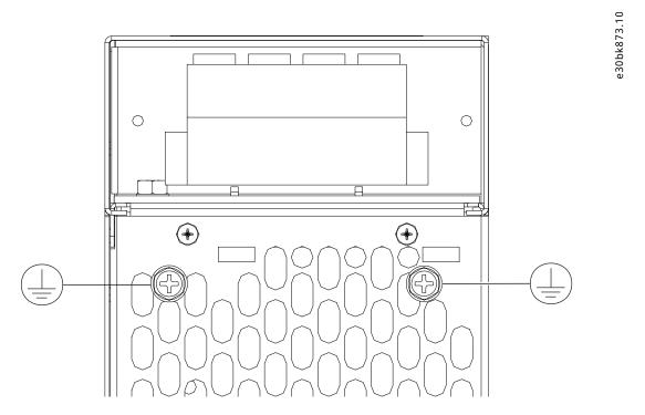
Figure 8: Positioning of Grounding Terminals for 35 A and 55 A filter modules
