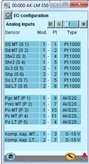
The setup of the analog inputs appears as it is supposed to according to the wiring made.
