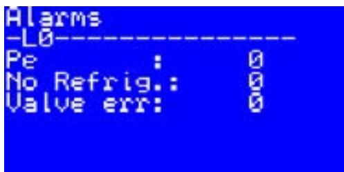
The active alarms screen displays details of the currently unacknowledged alarms. If more than one alarm has not been acknowledged, pressing the up or down buttons scrolls between them.
