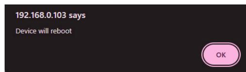
1.6 This operation takes 2-3 minutes long to be completed. Main rectangular horizontal LED in the X-Gate front will stay fixed and blink through different colours as yellow, green and purple colours. When the LED starts to keep blinking only green, the soft reset process is finished.
