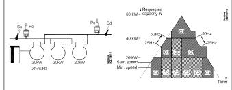
As the variable part of the speed controlled compressor is smaller than the following compressor steps the capacity curve will have some holes that can not be filled out by the variable capacity.
