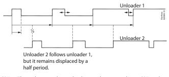
CRII 6: The pulse signal can also be used to control one CRII with three unloaders (6-cylinder version). The compressor signal is connected to one relay output.
