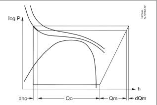
The function also increases the load on the compressor motor as pressure increases. Power consumption increases to Qm+dQm.
