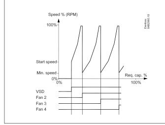
The controller starts the frequency converter and increases the speed of the first fan.
