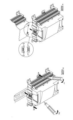
When the two snap catches for the DIN rail mounting are in the open position, the module can be pushed into place on the DIN rail – regardless of where the module is on the row.
