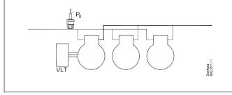
An error in the controlling sensor will mean that regulation continues with fx. 50% cutin in daily operation and fx. 25% cut-in at night, but for a minimum of one step.
