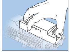
Press in the plate on the left-hand side of the light-emitting diodes and the plate on the right-hand side for the red address changers.
