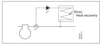
The heat recovery function can be used on the installation when you want to make use of warm gas for heating purposes. When the function is activated the reference for the condenser temperature will be raised to a set value. If the controller must also activate a pump and/or a valve, a relay must be selected for the function.
