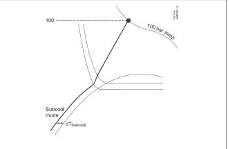
The controller is pre-programmed to follow the optimal COP from the pressure/enthalpy chart. The top point is defined at 100 bar, 39°C. (Optimal theoretical COP is achieved at the curve that passes through 100 bar and 39°C. The point of intersection can be changed by setting a value other than the default). Regulation will now follow the set reference curve, but will never
