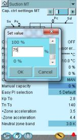
If you need to manually adjust the capacity of the compressors, you can use the following procedure:
