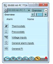
All the defined general functions are shown in overview display 2. In addition to always being shown in display 2, functions can be selected to be shown in display 1. Individual functions can be selected for display in display 1 via the "Show in overview display" setting.
