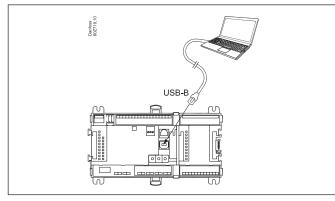
The controller must be switched on first and the LED "Status" must flash before the Service Tool program is started.
