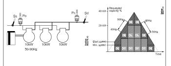
As the variable part of the speed controlled compressor is bigger than the following compressor steps, the capacity curve will be without holes.
