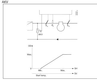
Four values are adjusted -- a start value for the Sd temperature, min. and max. values for overheating and a period time for the AKV valve.
