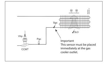
The pressure in the gas cooler is controlled by the valve CCMT valve with stepper motor can be used.
