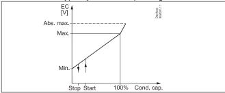
If the Sgc temperature exceeds the defined "Absolute Max Sgc temperature", the output voltage will be increased to the EC absolute maximum value.
