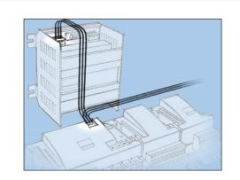
The controller has to be remote-monitored via a network. In this network we assign address number 3 to the controller. The same address must not be used by more than one controller in the same network.
