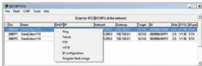
Figure 3: CHIPtool with a list of all available SonoCollect 110 in the local network
