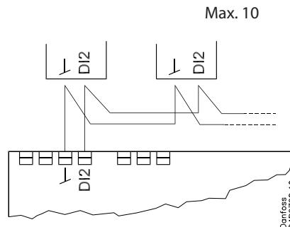
The following controllers can be connected up in this way:
