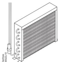
The condenser sensor is used to protect the compressor against high pressure when the condenser is blocked or the condenser fan fails.
