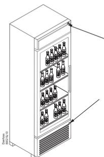
The ambient light sensor is used to detect opening hours of the shop.
