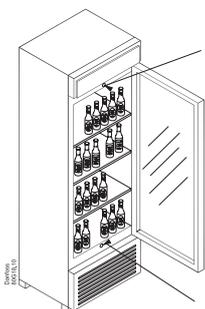
The door sensor is used to detect buying activity and to stop the fan when the door is opened.
