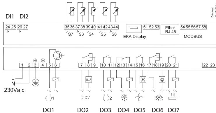
In application 1, the compressors are controlled sequentially. Compressor 1 is first in and last out.
