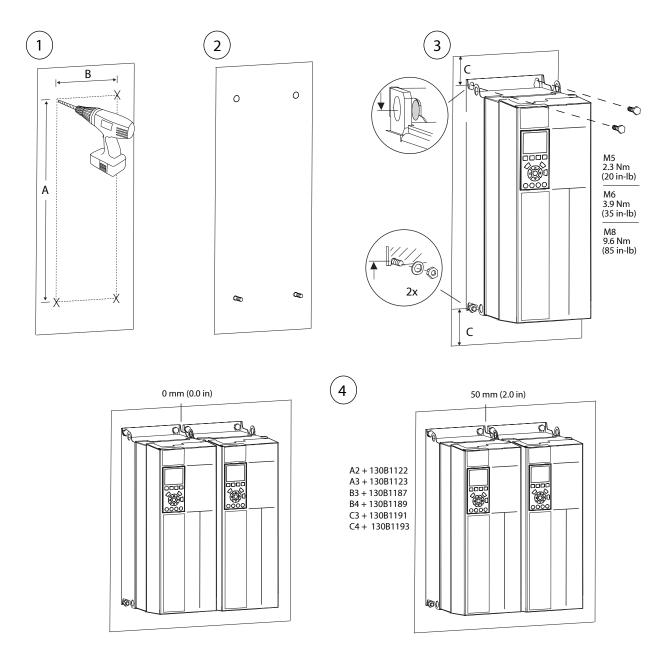
Figure 3: Wall-mount Installation
