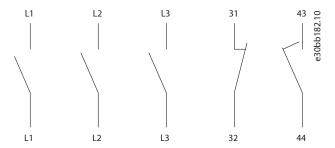
Figure 9: Terminal Connections for A5, B1, and B2
