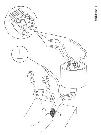
Figure 11: Installing a Category C1 Filter
