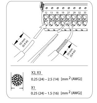
Figure 12: Accessing the Control Terminals
