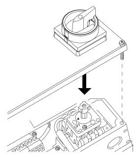
Figure 8: Location of Mains Switch (Enclosure Size A5)
