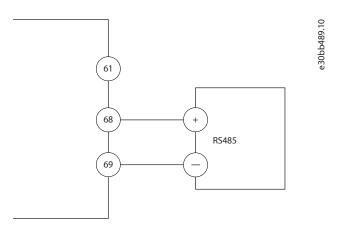
Figure 14: Serial Communication Wiring Diagram
