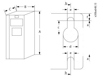
Figure 1: Top and Bottom Mounting Holes
