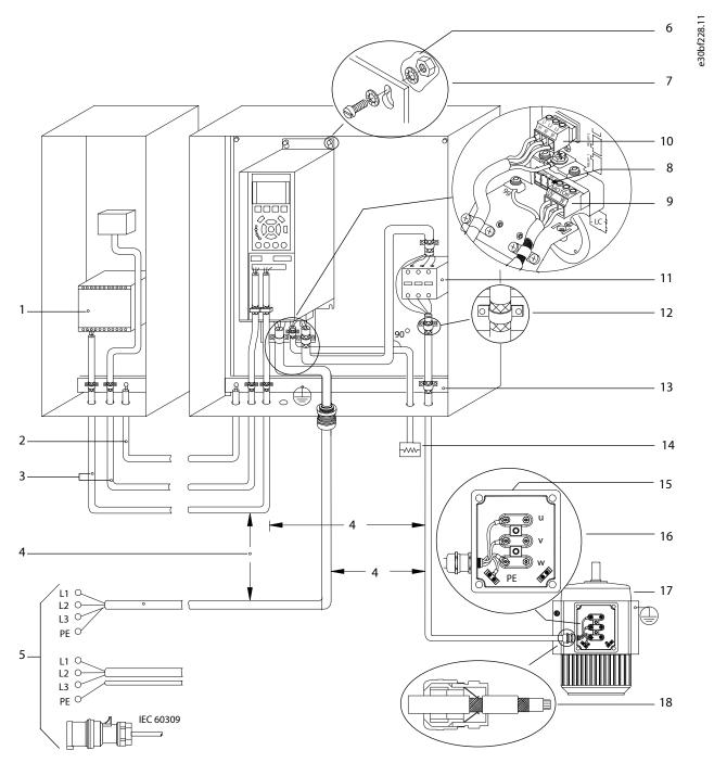
Figure 4: Example of Proper EMC Installation
