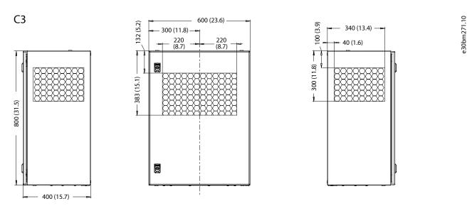
Figure 6: Allowed Ventilation Openings for C3 Enclosures as Tested for UL61800-5-1 Compliance
