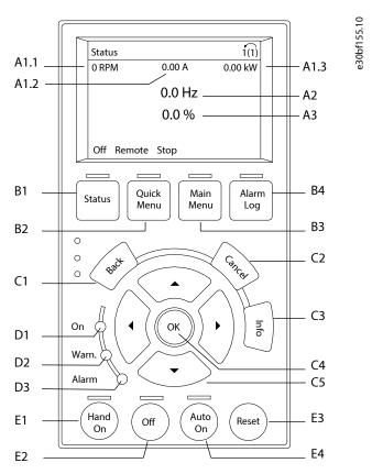
Figure 16: Graphical Local Control Panel (LCP)
