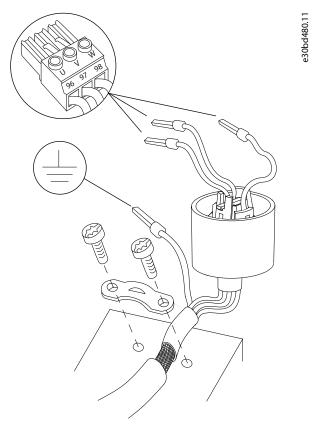
Figure 11: Installing a Category C1 Filter
