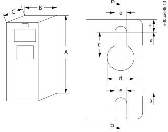
Figure 1: Top and Bottom Mounting Holes
