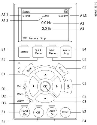
Figure 16: Graphical Local Control Panel (LCP)
