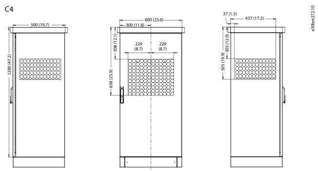
Figure 7: Allowed Ventilation Openings for C4 Enclosures as Tested for UL61800-5-1 Compliance
