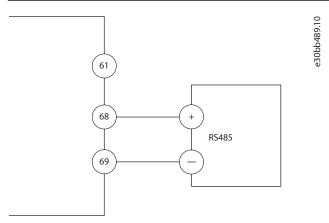
Figure 14: Serial Communication Wiring Diagram
