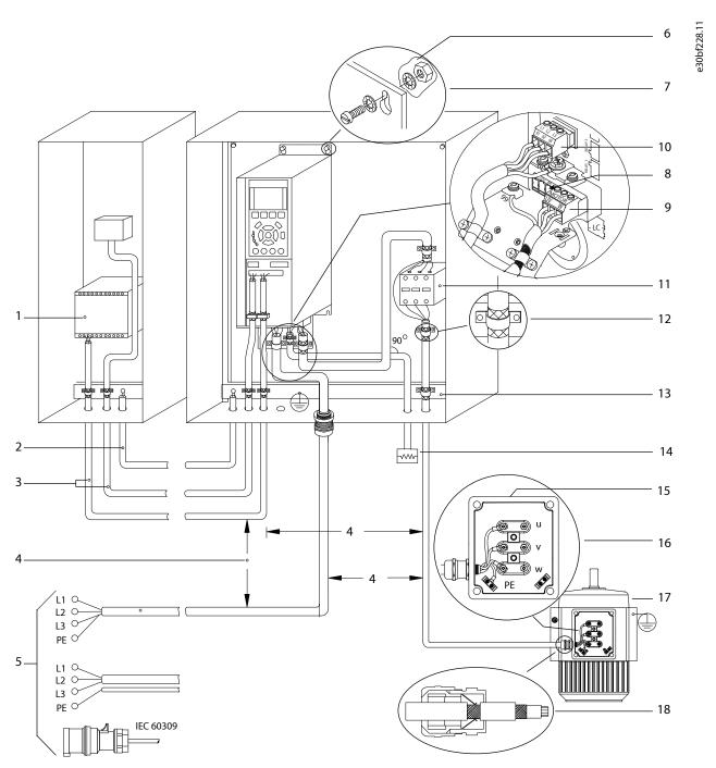
Figure 4: Example of Proper EMC Installation
