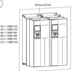
Figure 3: Wall-mount Installation
