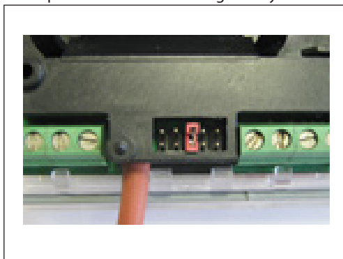
Fig. 5.1 Jumper setting for test mode
