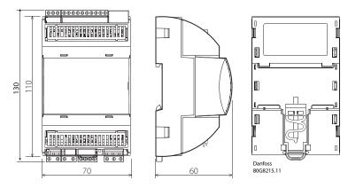
For DIN rail mounting only (IP20)
